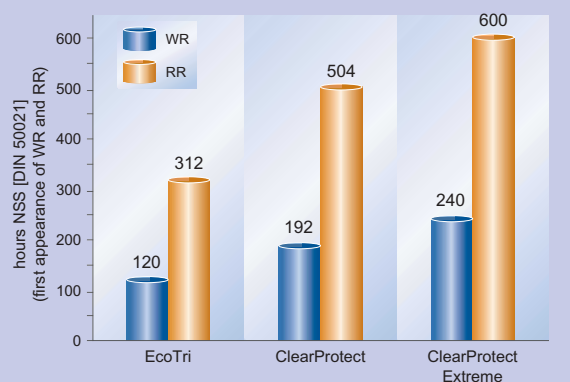
Corrosion Protection (DIN 50021 SS) of EcoTri, ClearProtect and ClearProtect Extreme on cyanide-free alkaline zinc coating Protolux 3000 (8 µm) in rack application (right) and barrel/basket application (above)
