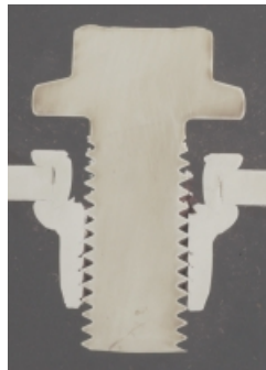
Standard Inserts (9498 series) Joint Failure Mode = Thread Stripping Insert Needs Removal & Replacement
