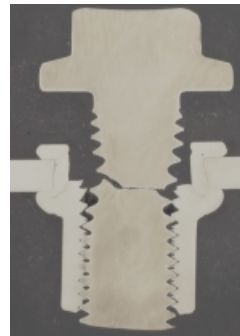
High strength Hexsert® Inserts (39301 series) In Over Torque Joint Failure Mode = Bolt Breakage Insert Not Damaged
