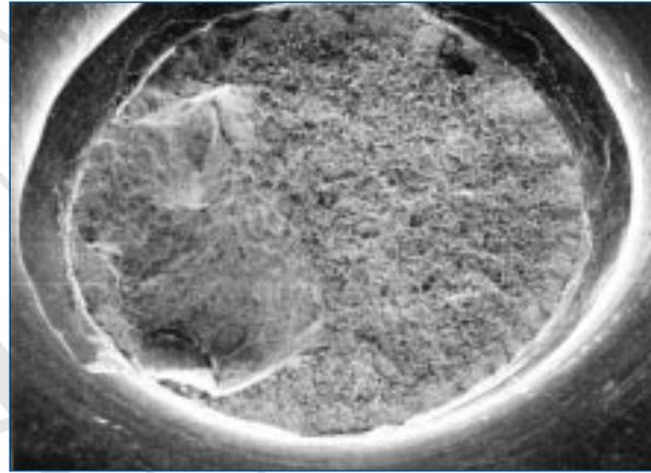
**A typical hydrogen embrittlement fastener fracture.**
